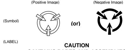
CONTAINS PARTS AND ASSEMBLIES SUSCEPTIBLE TO DAMAGE BY ELECTROSTATIC DISCHARGE (ESD)
